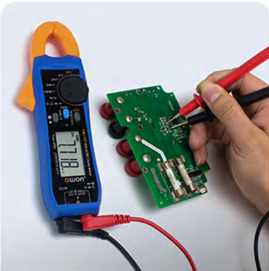
Circuit board resistance measurement
