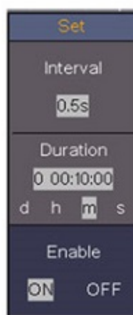
The data logging function of multimeter
